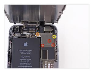
Incorrect placement of these screws during reassembly will cause permanent damage to your iPhone's logic board.
