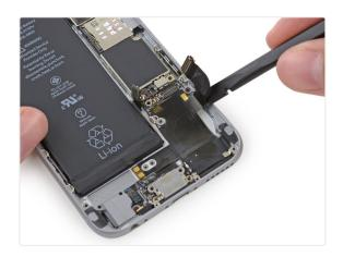
• Use the flat end of a spudger to begin peeling the Lightning connector assembly up from the rear case.
