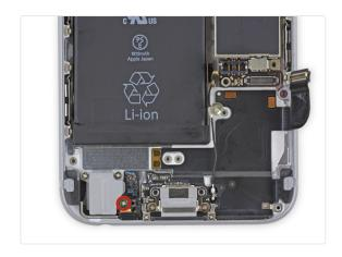
• Remove the single 3.6 mm Phillips #00 shoulder screw from the microphone brace.
