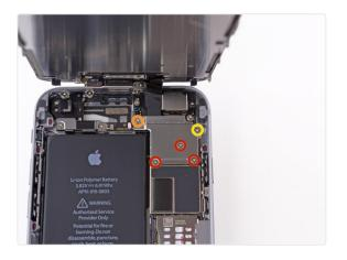
Incorrect placement of these screws during reassembly will cause permanent damage to your iPhone's logic board.
