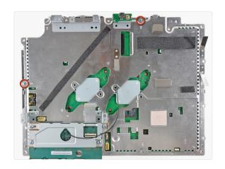
• Remove the two 8.3 mm #0 Phillips screws securing the two halves of the motherboard together.
