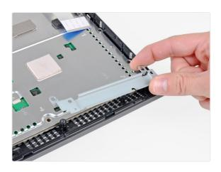
• Remove the control board bracket.
