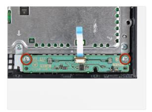
• Remove the control board and its attached cable from the PS3.
