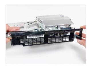
• Remove the rear cover from the logic board assembly.
